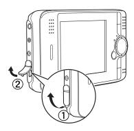
3 Connect the small end of the USB cable to the P-4000.
