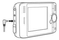
2 Connect the USB cable to your computer. Then open the USB connector cover and connect the other end of the USB cable to the P-4000.
