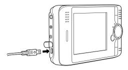
4 Connect the other end of the cable to the EXT I/F connector on the printer.
