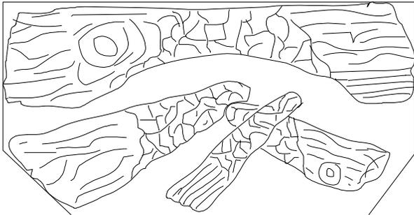
3. Gently remove the ember material from the plastic bag. Place a single line of embers on burner as shown beside.
