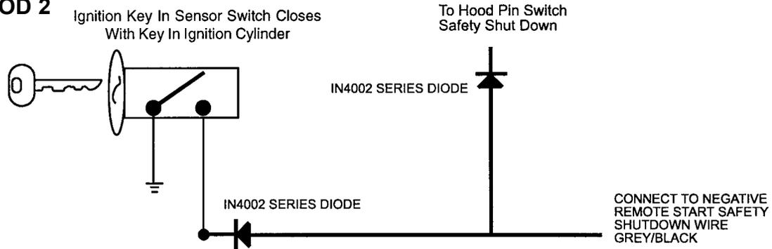
To connect to the key in sensor circuit as shown for method 2:
