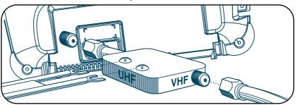
If your antenna system has two sets of twin 300-ohm leads, you must obtain a combiner (available at your local electronics store). Place one set of twin leads underneath the screws on the combiner and tighten the screws. Do the same with the other set of twin leads. Press the cable from the combiner onto antenna terminal on the back of your TV.
