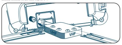
If your cable system requires you to use a converter box for all channels, connect the incoming cable to the IN terminal on the converter box. Connect another cable between the OUT terminal on the converter box and the antenna terminal on the TV. You will need to keep your TV tuned to channel 3 or 4 and change channels using the converter box.
