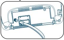
If your antenna ends in a single coaxial lead, simply press or screw the cable onto the antenna terminal on the back of your TV.
