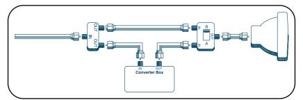
When the A/B switch is in the A position, you need to change channels on the converter box (and your TV should be tuned to channel 3 or 4); when the A/B switch is in the B position you can change channels on the TV.
