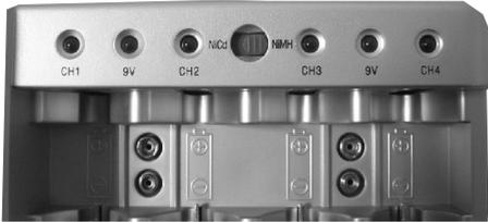
3. Slide the Battery Type Switch to select the correct type of battery. For Nickel-Cadmium batteries, set the Battery Type Switch to the NiCd position. For Nickel-Metal Hydride batteries, set the Battery Type Switch to the NiMH position. See illustration.
