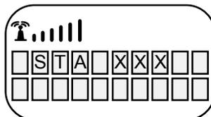
**Figure 3.6.21 LCD Message of Subscribed GDC-335H (GAP) and GDC-340H (GAP)**
