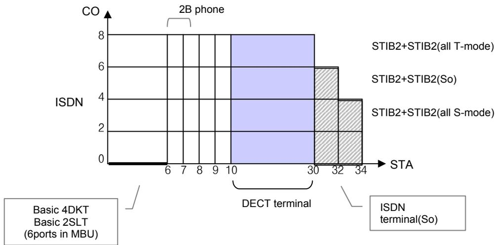
1) GDK-20W System Configuration Chart with STIB/STIB2(ISDN Board)
