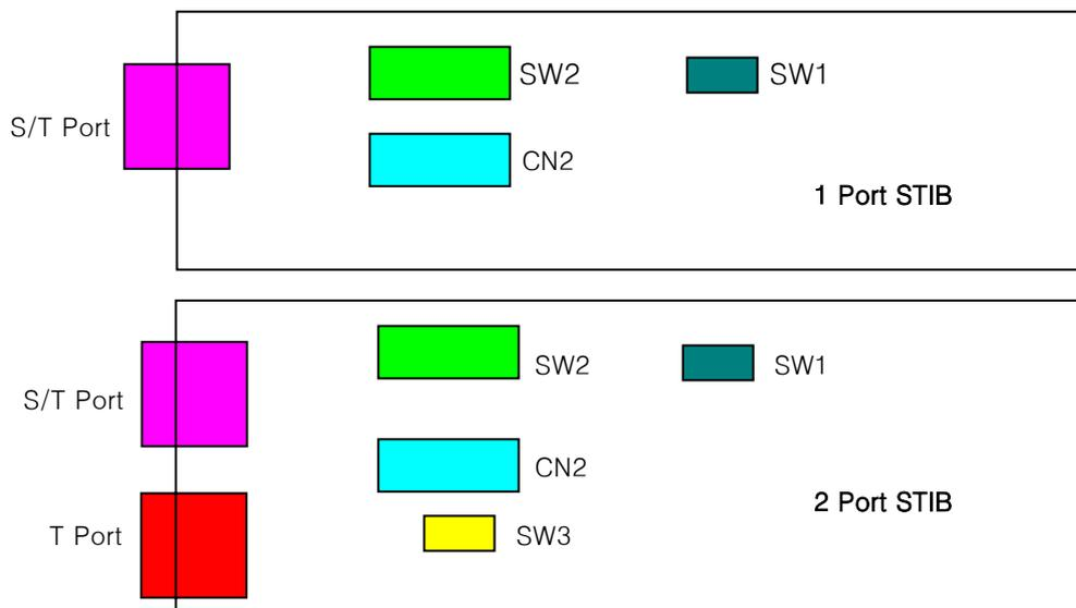
Figure 3.4.8 Switches and connector for the STIB
