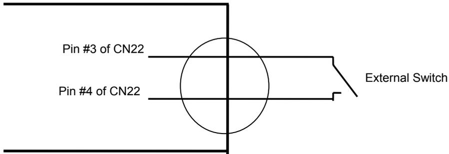
Figure 3.5.3 External Switch Wiring Example
