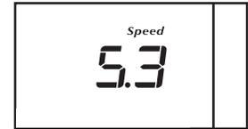
If one of the 1-Step Speed buttons is pressed, the walking belt will gradually increase in speed until it reaches the selected speed setting.
