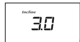
If one of the 1-Step Incline buttons is pressed, the incline will gradually increase until it reaches the selected incline setting.
