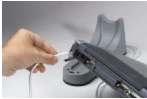
Figure 18. Connecting the USB Connector to the USB Port
