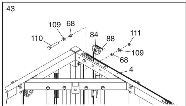
44. Route the High Cable (88) over a Small Pulley (84) and down through the Left Top Frame (4). Attach the Pulley inside the Left Top Frame with an M10 x 65mm Bolt (110), two M10 Washers (109), two 1/2" Spacers (68), and an M10 Nylon Locknut (111).
