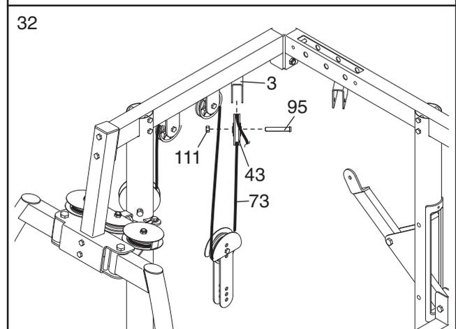
33. Wrap the Butterfly Cable (73) over a Pulley (43). Attach the Pulley to the Center Top Frame (6) with an M10 x 45mm Bolt (95) and an M10 Nylon Locknut (111).
