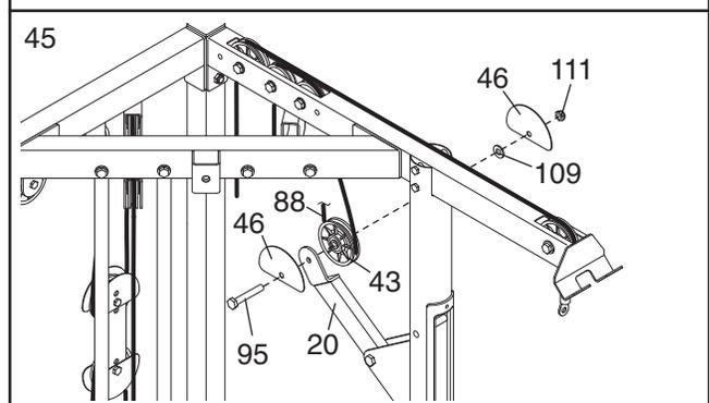
46. Wrap the High Cable (88) over a Pulley (43). Attach the Pulley to the Left Top Frame (4) with an M10 x 45mm Bolt (95) and an M10 Nylon Locknut (111).
