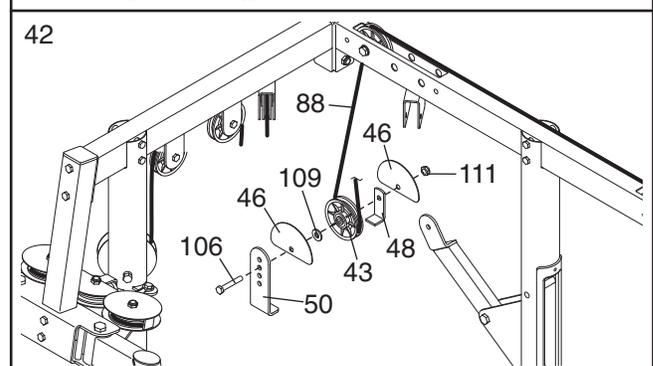
43. Route the High Cable (88) up through the Left Top Frame (4) and over a Small Pulley (84). Attach the Pulley inside the Left Top Frame with an M10 x 65mm Bolt (110), two M10 Washers (109), two 1/2" Spacers (68), and an M10 Nylon Locknut (111).
