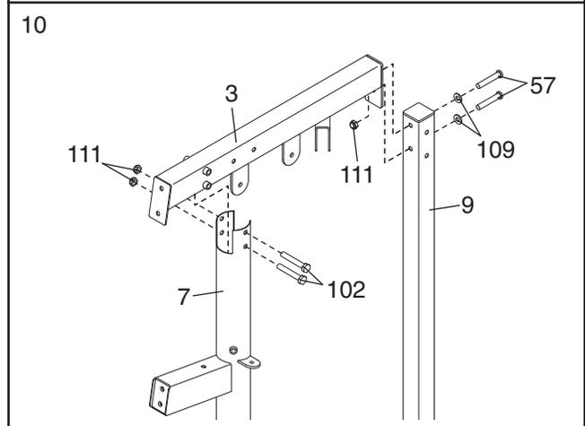
Attach the Right Top Frame (3) to the Right Upright (7) with two M10 x 90mm Bolts (102) and two M10 Nylon Locknuts (111). **Do not tighten the Nylon Locknuts yet.**
