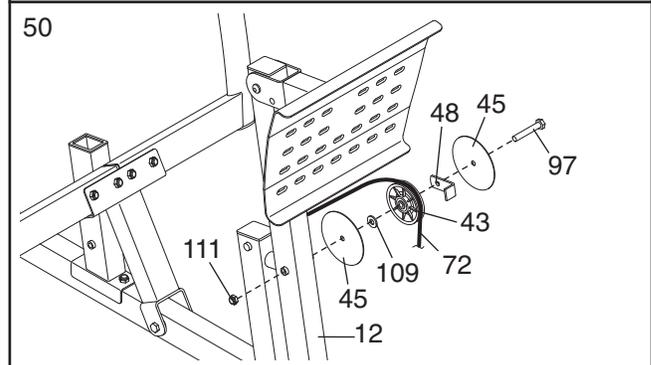
51. Wrap the Press Cable (72) under a Pulley (43). Attach the Pulley, a Cable Trap (48), an M10 Washer (109), and two Finger Guards (45) to the Left Seat Upright (14) with an M10 x 120mm Bolt (97) and an M10 Nylon Locknut (111). **Make sure that the Cable Trap is oriented to hold the Cable in the groove of the Pulley.**
