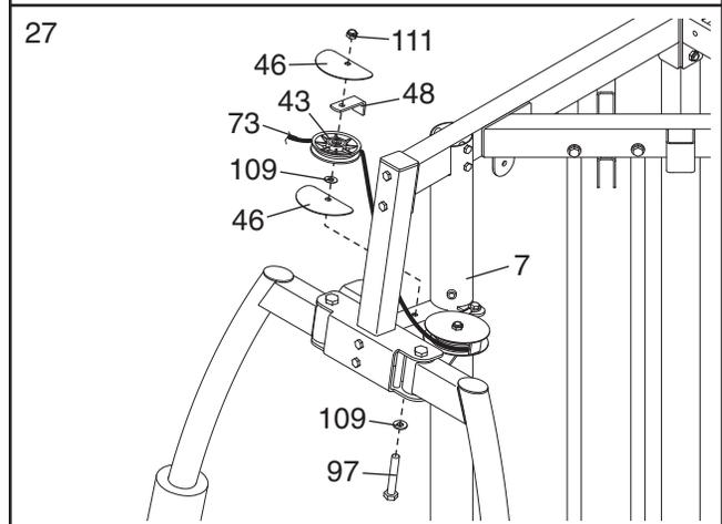
28. Wrap the Butterfly Cable (73) around a Pulley (43). Attach the Pulley, a Cable Trap (48), an M10 Washer (109), and two Finger Guards (45) to the Right Butterfly Arm (23) with an M10 x 50mm Bolt (106) and an M10 Nylon Locknut (111). **Make sure that the Cable Trap is oriented to hold the Cable in the groove of the Pulley.**
