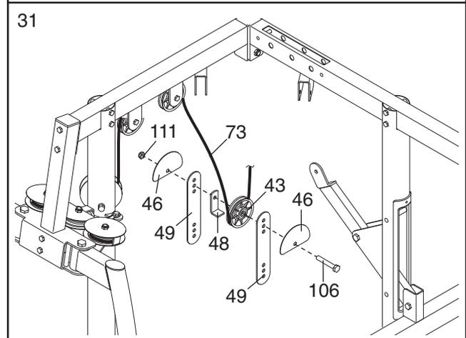
32. Wrap the Butterfly Cable (73) over a Pulley (43). Attach the Pulley to the Right Top Frame (3) with an M10 x 45mm Bolt (95) and an M10 Nylon Locknut (111).
