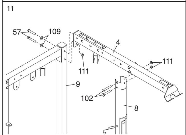
Attach the Left Top Frame (4) to the Left Upright (8) with two M10 x 90mm Bolts (102) and two M10 Nylon Locknuts (111). **Do not tighten the Nylon Locknuts yet.**
