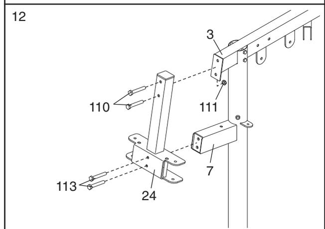
Attach the Butterfly Frame (24) to the Right Upright (7) with two M10 x 35mm Screws (113). **Do not tighten the Screws yet.**
