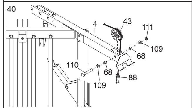
41. Route the High Cable (88) over a Pulley (43) and down through the Left Top Frame (4). Attach the Pulley inside the Left Top Frame with an M10 x 65mm Bolt (110), two M10 Washers (109), two 1/2" Spacers (68), and an M10 Nylon Locknut (111).
