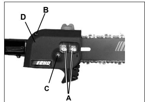
5. Install chain on guide bar with cutters on top of bar facing toward bar tip.
