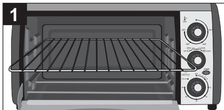
Place the Wire Rack in the desired slot.
