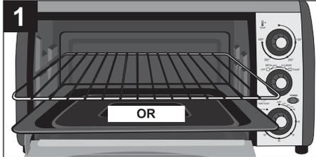
Place the Wire Rack (if using a separate oven-safe container) or the Baking Pan (if baking directly on it) in the desired slots depending on the food to be cooked.
