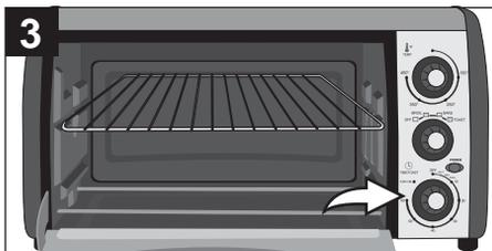
Rotate the TIMER knob to 10 minutes to preheat the oven. When the oven is done preheating, place the food in the oven and rotate the TIMER knob to the desired baking time or counter clockwise to the STAY ON position if you want to control cooking time or need to cook your food longer than 60 minutes.
