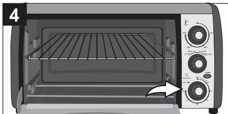
The oven is done cooking when the TIMER knob reaches OFF and a bell rings. You can also rotate the TIMER knob to OFF to stop cooking. If the STAY ON feature has been selected, the toaster oven must be shut off manually by turning the TIMER knob to the OFF position. Remove the oven-safe container or included Baking Pan using the Handle as shown on page 4.
