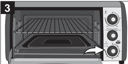
3 Place the food on the Wire Rack and rotate the TIMER knob to the desired broiling time or counter clockwise to the STAY ON position if you want to control cooking time or need to cook your food longer than 60 minutes.
