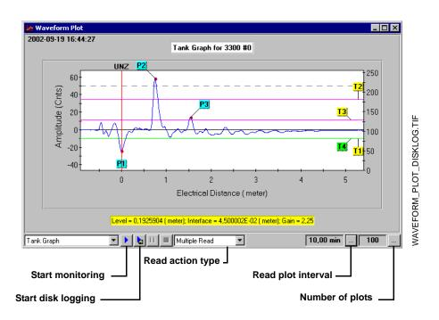
Figure 6-3. Disk logging Waveform plot
