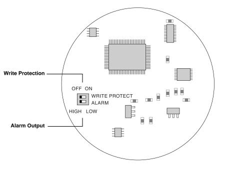
To set the Alarm and Write Protect switches do the following:
