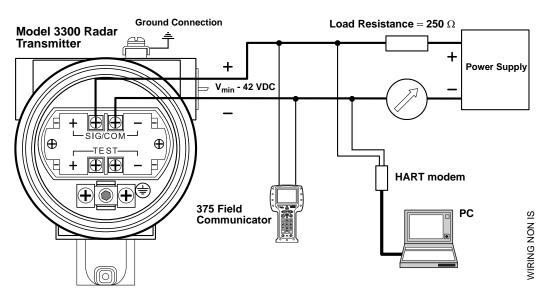
For HART communication a minimum load resistance of 250 Ohm within the loop is required. For maximum load resistance see Figure 3-12 (Explosion/Flame Proof) and Figure 3-13 (Non-hazardous installations).
