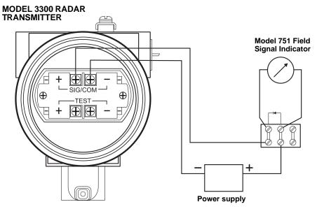
Figure 3-20. Alternative wiring diagram for 3300 transmitter with 751 Field Signal Indicator
