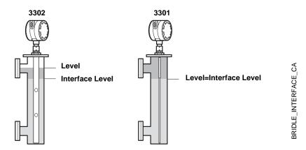
Coaxial, Rigid twin, Flexible twin and Rigid Single lead probes can be used for measuring interfaces. The coaxial probe is the preferred choice for clean liquids and when the bridle is not fully immersed. In applications with a fully immersed probe, the twin lead probes are recommended for nozzle installations, and the rigid single lead probe is best for bridle mounting.
