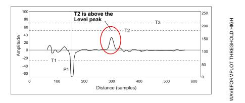
If there are disturbing objects in the tank the threshold must be carefully set in order to avoid locking on the wrong amplitude peak. In Figure 6-11 the transmitter has locked on a peak above the actual product surface, i.e. a disturbance was interpreted as the product surface, whereas the actual product surface was interpreted as an interface or the probe end.
