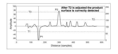
Figure 6-12. Waveform plot after threshold T2 was adjusted
