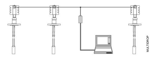
The poll address can be changed by using a 375 Field Communicator or by using the Rosemount Configuration Tools software.
