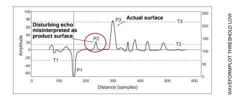
Figure 6-11. Example 2: amplitude threshold T2 is too low.
