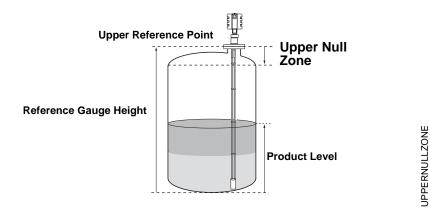
Figure 6-9. Identifying the Upper Null Zone in the RCT Waveform Plot
