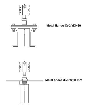
Avoid disturbing EMC environment near the tank. Installation in metallic tank is recommended.
