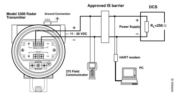
For HART communication a minimum load resistance of 250 Ohm within the loop is required. For maximum load resistance see Figure 3-14.
