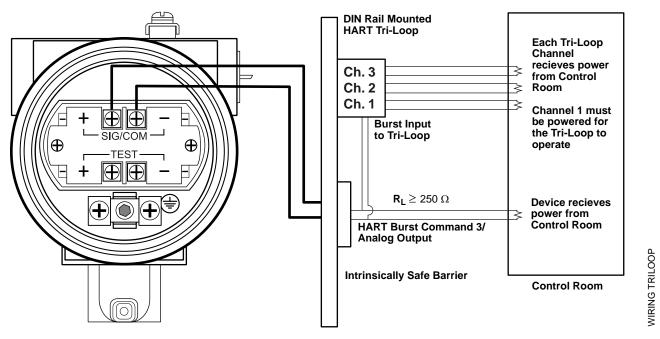
Configure Channels 1, 2, and 3 to reflect the units as well as Upper Range Values and Lower Range Values for your secondary, tertiary and fourth variables (variable assignment is configured in the Model 3300). It is also possible to enable or disable a channel from this menu. See "Special Functions" on page 4-24 for further information on how to install a Tri-Loop.
