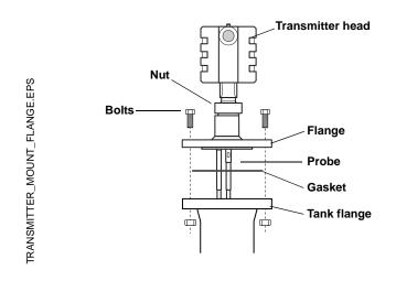
Figure 3-10. Tank connection with loose flange ("plate design").
