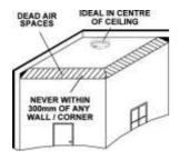
Place the mounting plate on the ceiling/wall and mark the screw holes. Drill with a suitable drill bit, insert the screw plugs and screw the plate into position. Simply slide the alarm into position on the mounting plate (this also activates the battery connection).
