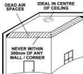
Alarms should be placed in accordance with the general guidelines shown in the diagram above. These recommendations are based on the problem of areas of "dead air" close to corners of rooms and apexes of ceilings, which could result in the prevention of smoke reaching the smoke detector
