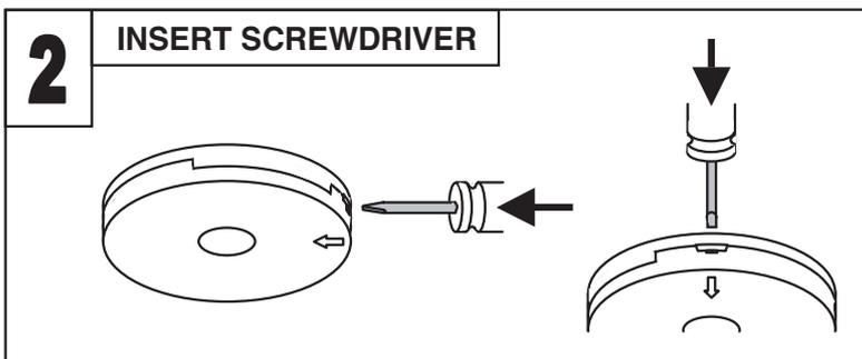
INSERT A FLAT-BLADED SCREWDRIVER HORIZONTALLY APPROX. 1cm INTO THE CENTRE OF THE REMOVAL SLOT
