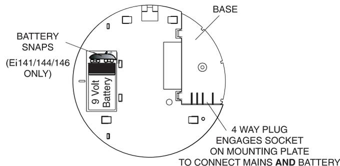
We recommend that the battery is replaced at least every three years for optimum performance.
