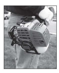
To avoid burns, always make sure that the muffler side of the engine is away from your body.
