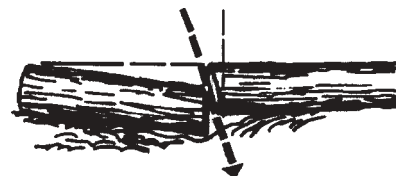
MAKE ANGLED CUT WHEN ONE SECTION MAY SETTLE AGAINST ANOTHER. KEEP BODY OUT OF BAR/CHAIN PATH!
