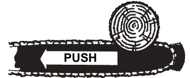
CUTTING ON TOP OF GUIDE-BAR PUSHES SAW TOWARD YOU
