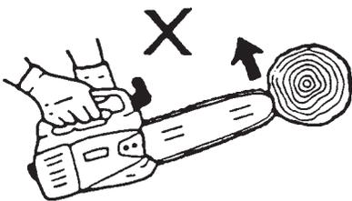
Improper thrust cutting.
