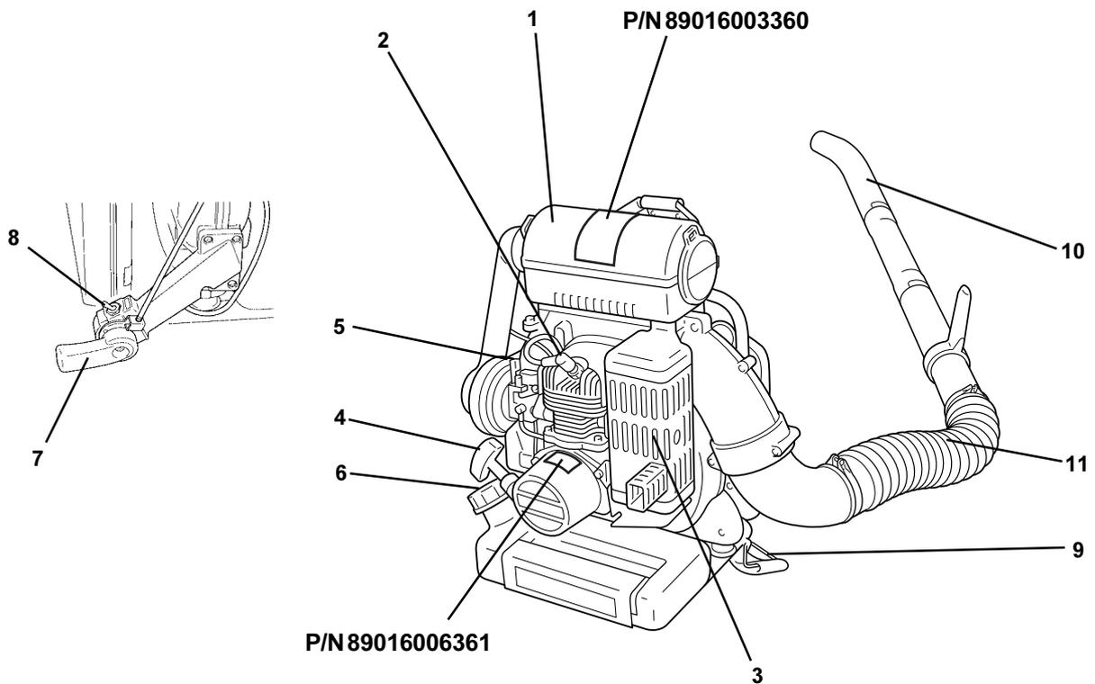
1. **AIR CLEANER** - Contains replaceable air filter element.
