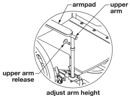
**⚠ WARNING: Ensure that arm is locked into place in level position before occupying or operating wheelchair.**
