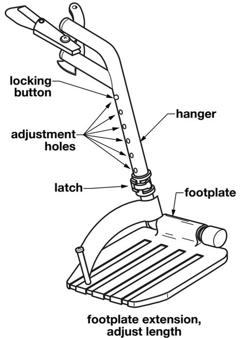
**⚠ WARNING: Ensure that footplates are securely fastened before occupying or operating wheelchair.**
