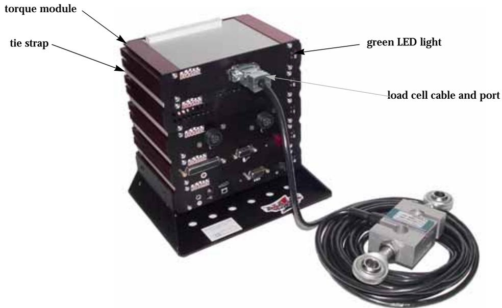
Figure 1-3: Attach Torque Module and Load Cell Cable
