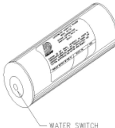
**Figure 2. Water Switch Location on Beacon**
