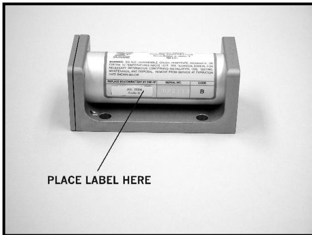
**Figure 21. RBB Label Placement**
