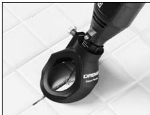
568 - Grout Removal Kit Four use on wall and floor grout • 30° angle for controlled cutting • Guides 180° apart to keep bit centered between tiles • Easy screw on mounting
