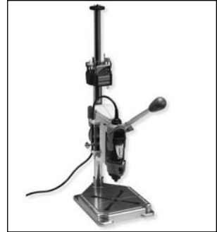
220 - Work Station For precision drilling, routing, grooving, 6" square work surface, 0" to 3" throat depth. Table slotted for guides, hold downs. Holds Model F013039519.
