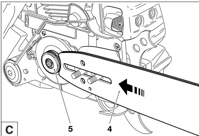
Position the guide bar (4) and push against the sprocket (5) as shown by the arrow.
