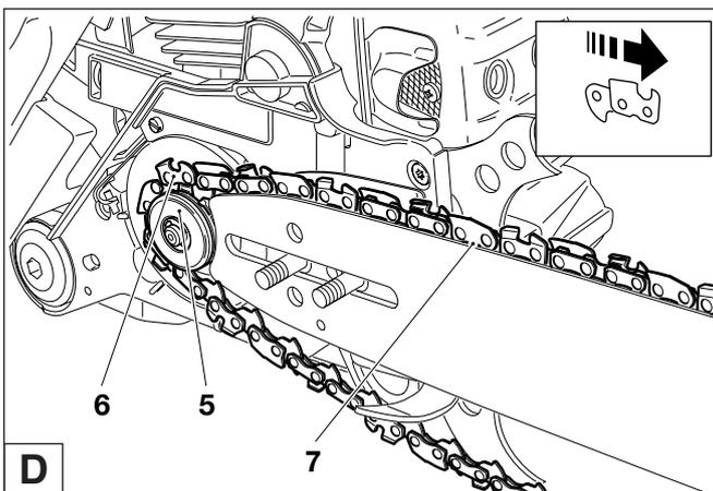
Lift the chain (6) over the sprocket (5). Using your right hand, guide the chain into the top guide groove on the guide bar (7).
