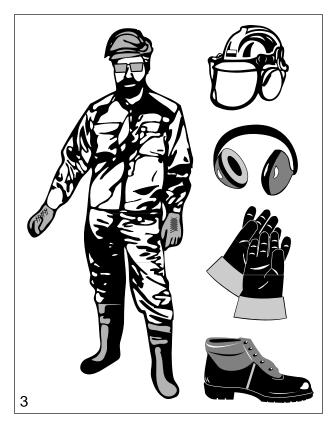
Good footing is most important in chain saw work. Wear sturdy boots with nonslip soles. Steel-toed safety boots are recommended.
