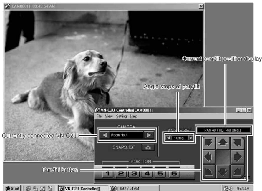
The connected VN-C2U angle steps of the pan/tilt can be changed using the right and left arrow buttons (← and →).
