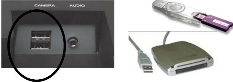
FIGURE 15 – CONNECTING A USB PERIPHERAL
