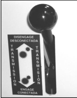
**Figure 20: Transmission Lever**
