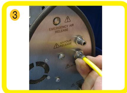
To remove **DRAIN** ( $\varnothing$  6mm) hose, press down the connector sleeve and pull the hose out.
