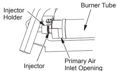
**Figure 26 - Injector Holder on Front Burner Tube**
