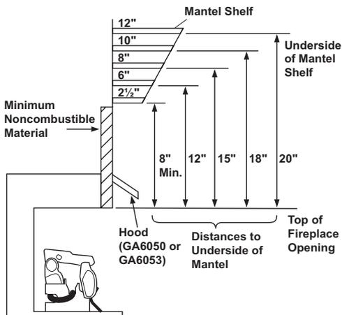
Figure 7 - Minimum Mantel Clearances When Using Hood
