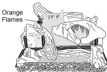
**Figure 24 - Incorrect Burner Flame Pattern**
