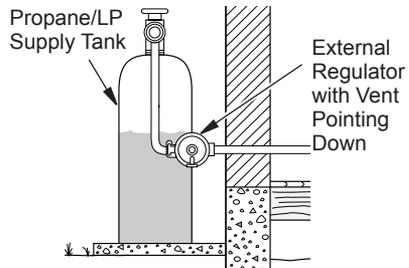
Figure 11 - External Regulator With Vent Pointing Down
