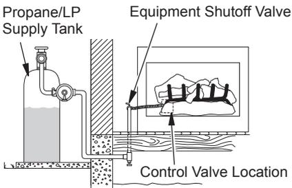
Figure 15 - Checking Gas Joints for Propane/LP Gas
