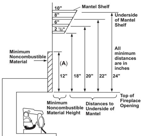
Figure 6 - Minimum Mantel Clearances Without Using Hood
