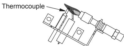
**Figure 21 - Correct Pilot Flame Pattern
