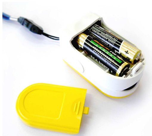
Figure 3 Installation des piles
