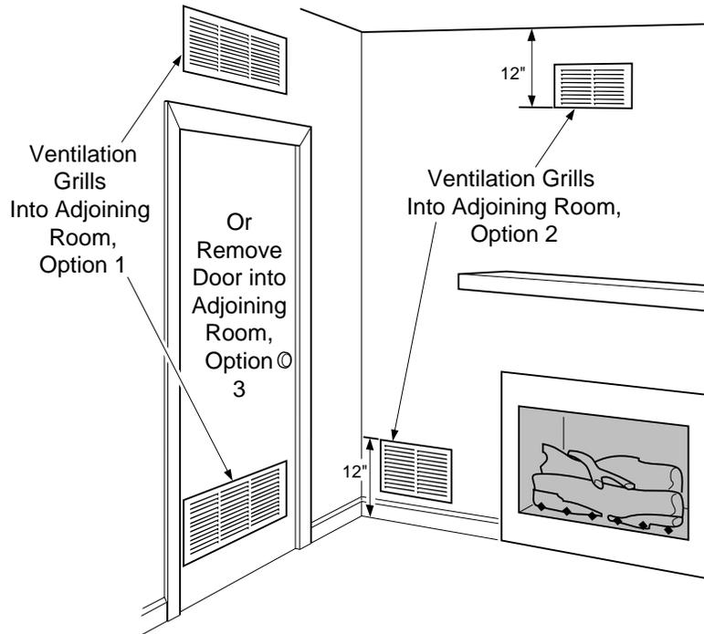
Figure 2 - Ventilation Air from Inside Building
