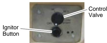
Figure 9 - Ignitor Button and Control Valve
