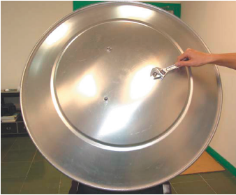
Figure 8 - Attaching Dome to Emitter
