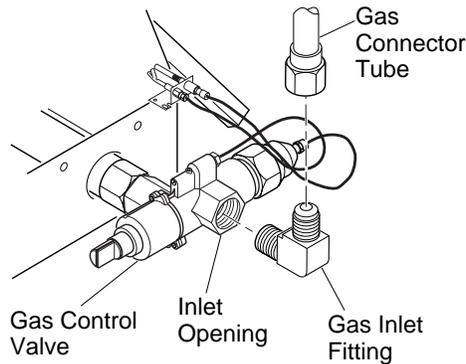
**Figure 13 - Installing Inlet Fitting and Gas Connector Tube**
