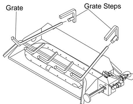
**Figure 18 - Installing Grate (Pan Material Not Shown)**
