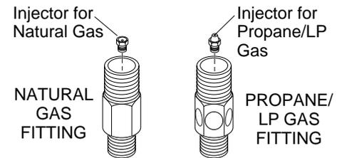
**Figure 15 - Burner Inlet Fittings with Injectors**
