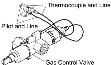
**Figure 12 - Gas Control Valve with Thermocouple and Pilot**
