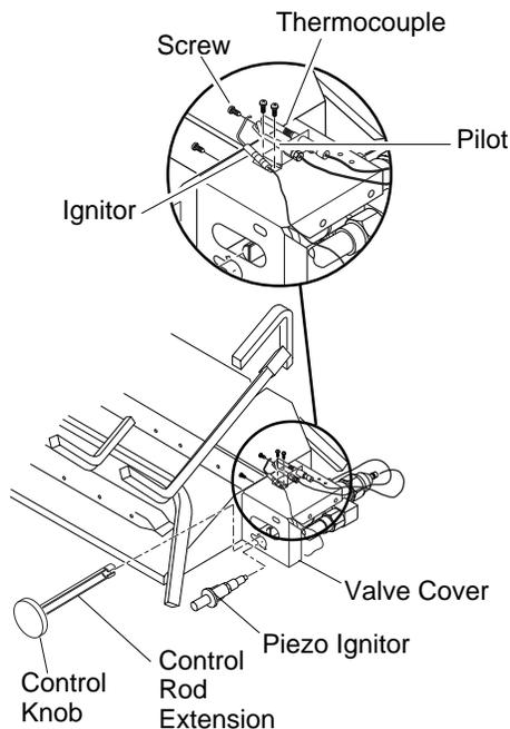
**Figure 14 - Installing Cover, Control Knob, and Piezo Ignitor**
