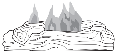
Figure 48 - Incorrect Burner Flame Pattern
