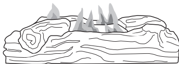
Figure 47 - Correct Burner Flame Pattern
