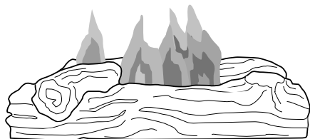
Figure 49 - Incorrect Burner Flame Pattern
