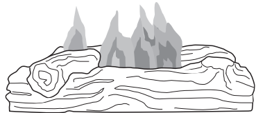
Figure 49 - Incorrect Burner Flame Pattern
