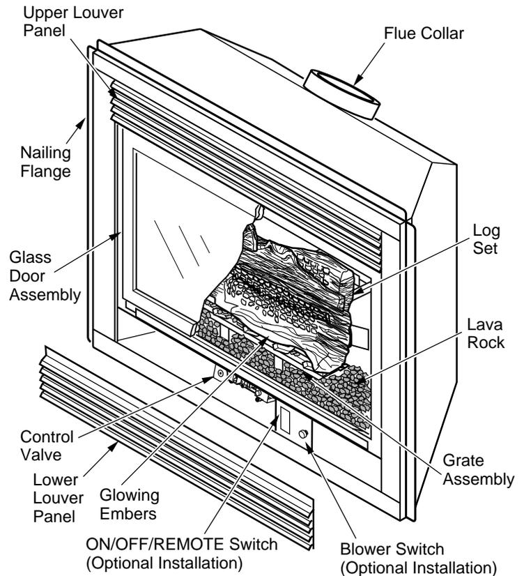
**Figure 1 - Victorian Direct-Vent Fireplace with Electronic Ignition**
