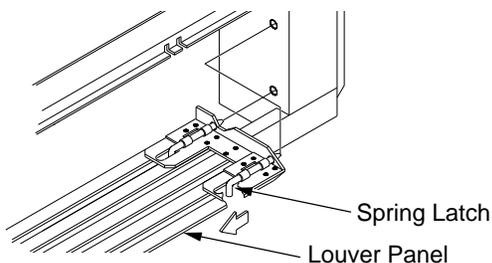
Figure 36 - Removing Louver Panel
