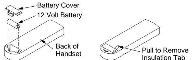
**Figure 48 - Installing Battery into Back of Handset**
