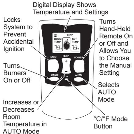
Figure 48 - Thermostat Hand-Held Remote Control Unit HRC200
