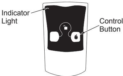
Figure 47 - On/Off Hand-Held Remote Control Unit HRC100
