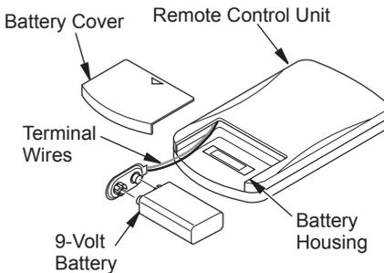
**Figure 40 - Installing Battery in Hand-Held Remote Control Unit**
