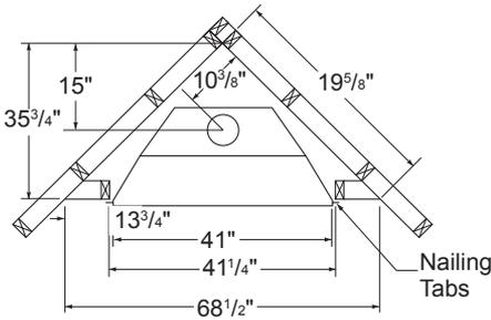
**Figure 5 - Framing Clearances for Corner Installation**
