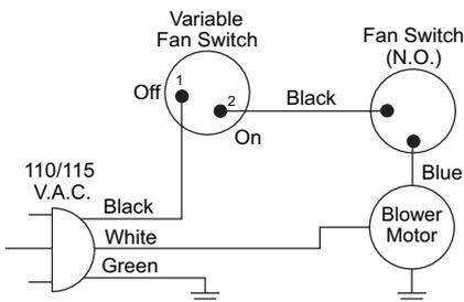
**Figure 30 - Blower Wiring Diagram for Thermostat-Controlled Models**
