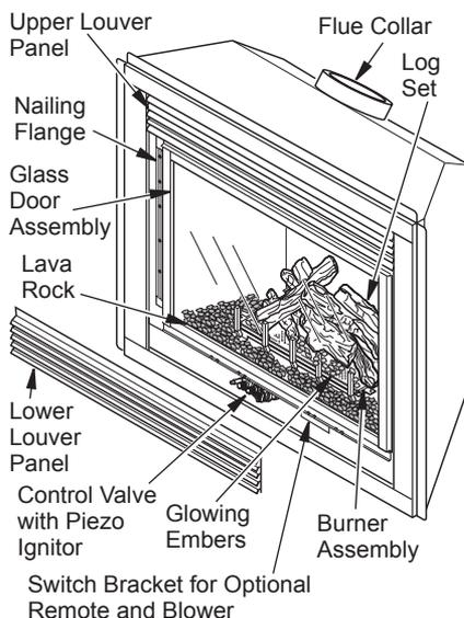
**Figure 1 - Direct-Vent Fireplace with Millivolt Ignition**
