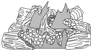
Figure 56 - Typical Flame Pattern
