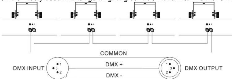
Termination reduces signal errors and to avoid signal transmission problems and interference. It is always advisable to connect a DMX terminal. (Resistance 120 ohm 1/4W) between pin2(DMX-) and pin3(DMX+) of the last fixture.
