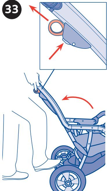
33. Hold the stroller as shown. Pull both orange triggers towards you. Push the brake lever with your foot and, at the same time, tilt the handle in a backwards direction. The stroller will begin to fold.
