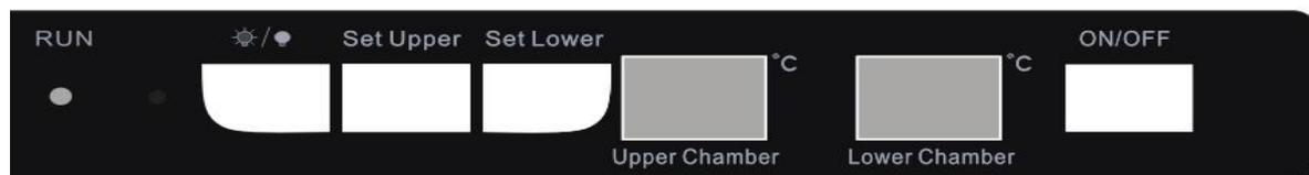
2. Set the desired cooling temperature by pressing the buttons adjacent to the « Set Upper / Set Lower » program. Each depression of the buttons will scroll through the available temperature settings (for each compartment) in increments of 1 degree. The temperature selected will flash in the LED display for approximately 5 seconds, then revert back to display the temperature of the internal cabinet.
