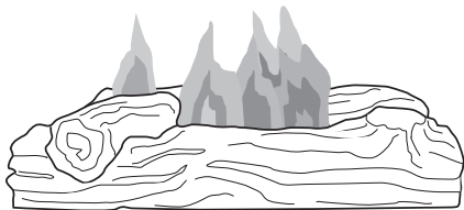
Figure 55 - Incorrect Burner Flame Pattern
