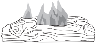
Figure 54 - Incorrect Burner Flame Pattern
