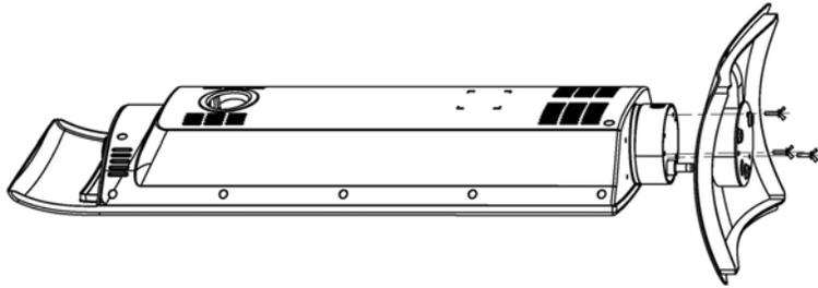
1. Unscrew the butterfly nuts from the bottom of the heater unit.
