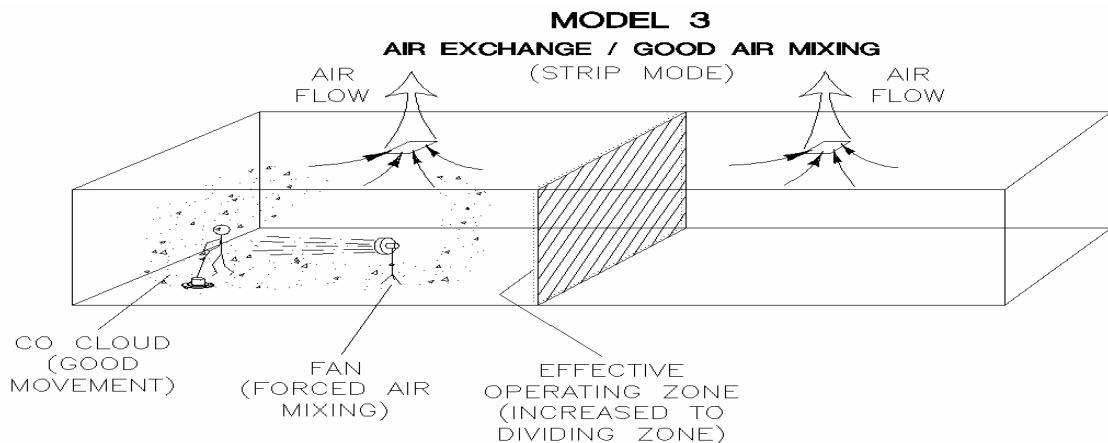
Notice the CO concentration and the Effective Operating Zone (Expanded to the Dividing zone) with air exchange and forced air mixing. The CO cloud is still concentrated on one side of the Dividing zone. Note the "Dividing Zone" shown above, this is the line where airflow changes direction. In Model 3, air changes are cut in  $\frac{1}{2}$  as little or no CO crosses the Dividing Zone to be exhausted.
