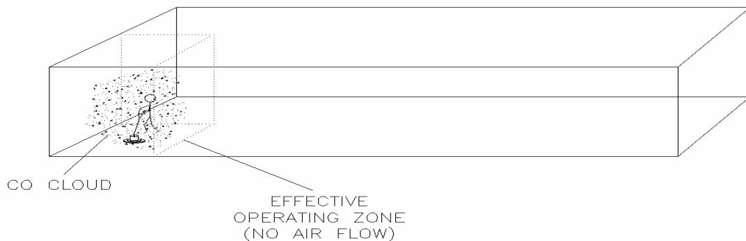
Stripping is quite a different type of operation than burnishing, and carries with it substantially more hazards, as stripping is a low movement operation compared to burnishing (less floor space for the same time). As shown in Model 1, the CO concentrations rise much quicker as the “Effective Operating Zone” is a very small area compared to the total building size.
