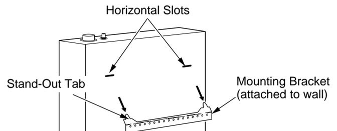
Figure 11 - Mounting Heater Onto Mounting Bracket
