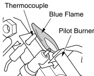
Figure 23 - Correct Pilot Flame Pattern
