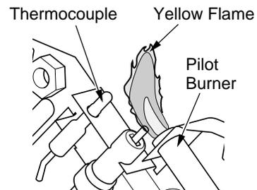
Figure 24 - Incorrect Pilot Flame Pattern
