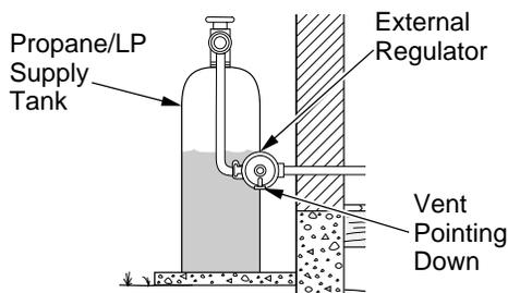
Figure 14 - External Regulator With Vent Pointing Down
