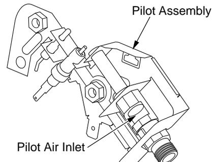
Figure 27 - Pilot Inlet Air (Propane/LP Pilot Shown)
