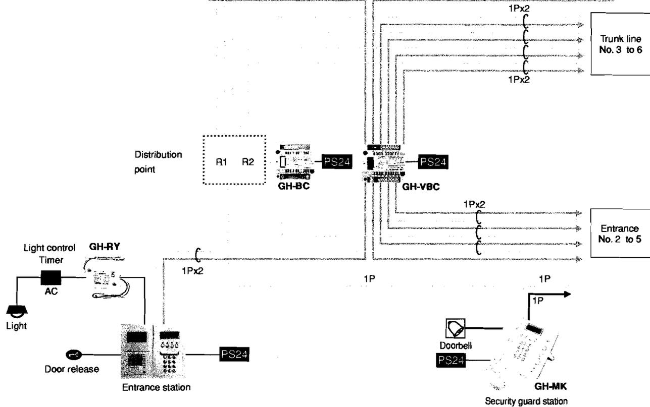
Cable: 1P x 2, 2-conductor cable solid copper & non-braided, polyethylene insulation
